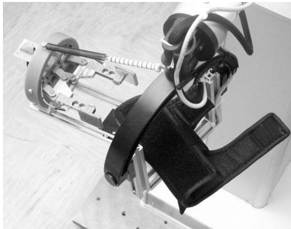
Figure 3. Grasp module consists of gimbal device, a wrist support splint and two-degrees of freedom mechanism for measuring the grasp force and for passive haptic rendering.
