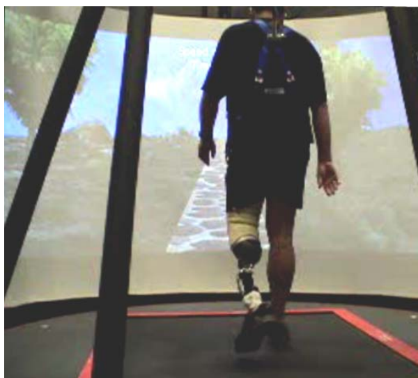
Figure 1. Participant walking on the CAREN system during the Continuous Road VE
