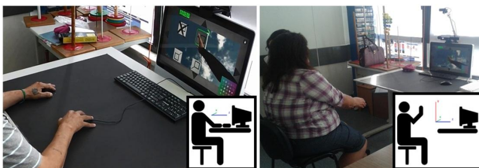
2-dimensional (a) and 3-dimensional (b) experimental setups. Inset images show the user's position relative to VR system and the allowed movements.
