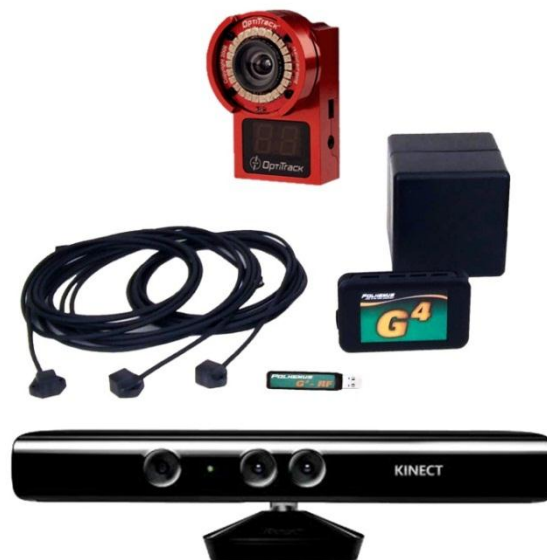
Tracking systems under study: optical; electromagnetic; and skeleton tracking.
