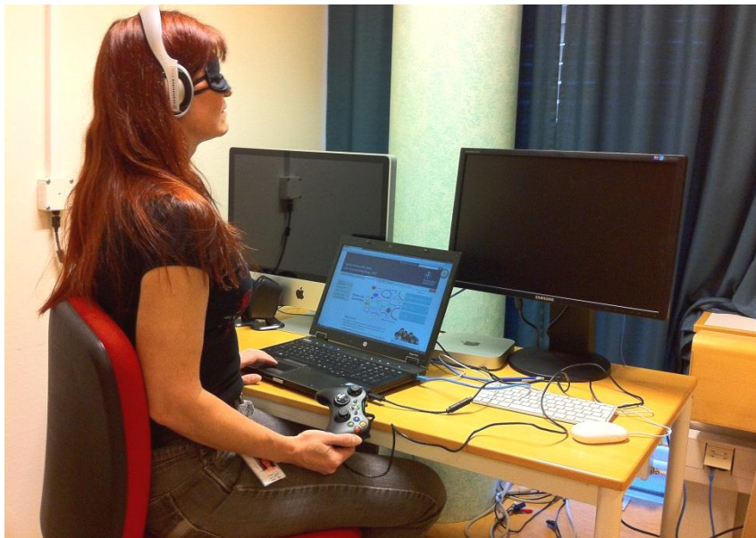
Test setup showing use of laptop touch pad for input and Xbox360 controller for output. Test subjects were blindfolded and wore ear protection.
