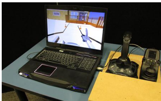
Experiment setup (left): Alienware laptop, gaming joystick, and PWC joystick; an outside view of the house environment used in our simulation (right).
