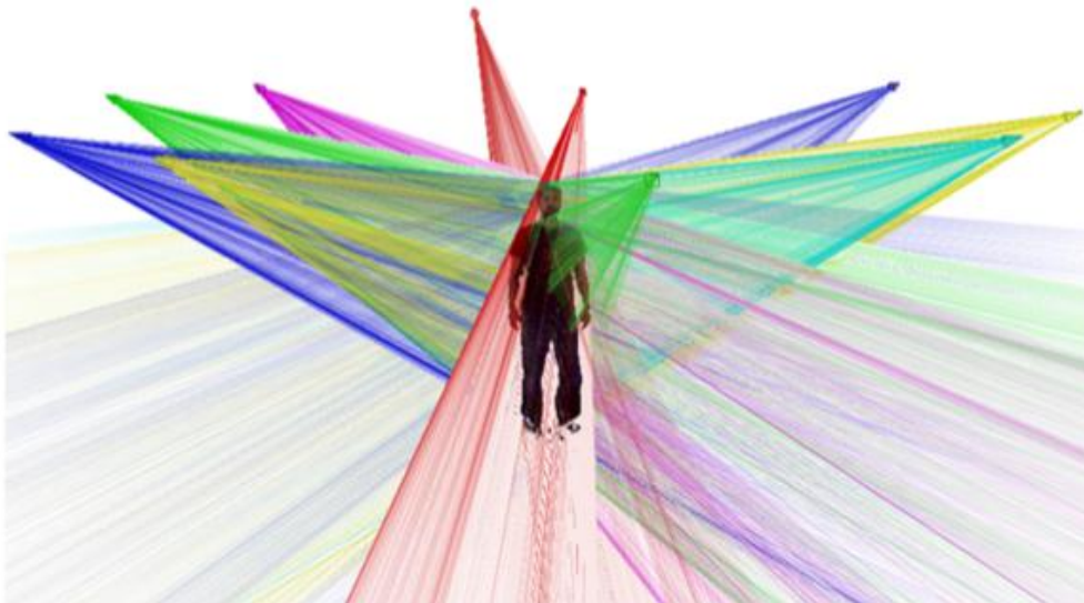
3D reconstruction of a human in our telepresence system, showing lines from each camera derived from silhouettes.
