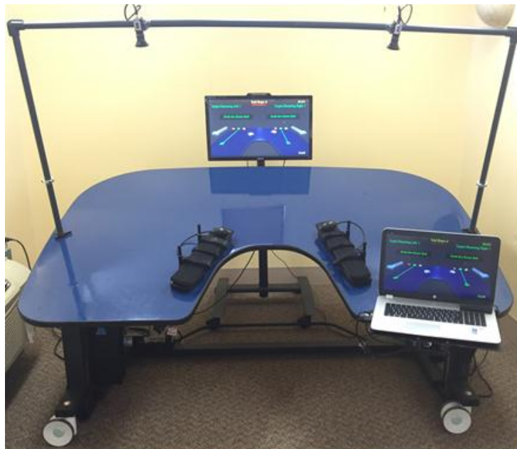
BrightArm Duo Table tilted upwards with two arm supports for user interaction and therapist laptop rendering Pick & Place game to the 27" monitor.
